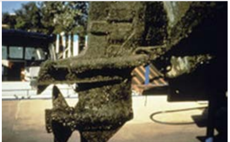
Photo: Zebra mussels covering a motor, Steve Kynock, Michigan Sea Grant, Bugwood.org
