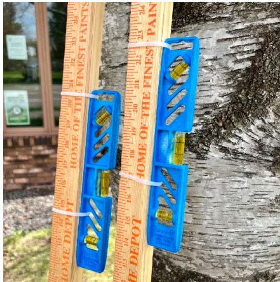
Step 1-2: Use zip ties to attach levels
